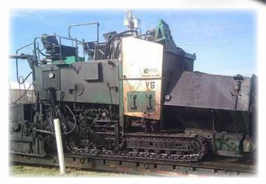
The pavers have air-cooled motors with small 5-gallon sumps, making this high-temperature application very difficult. A high-performance oil was needed to keep the pavers on the job.
